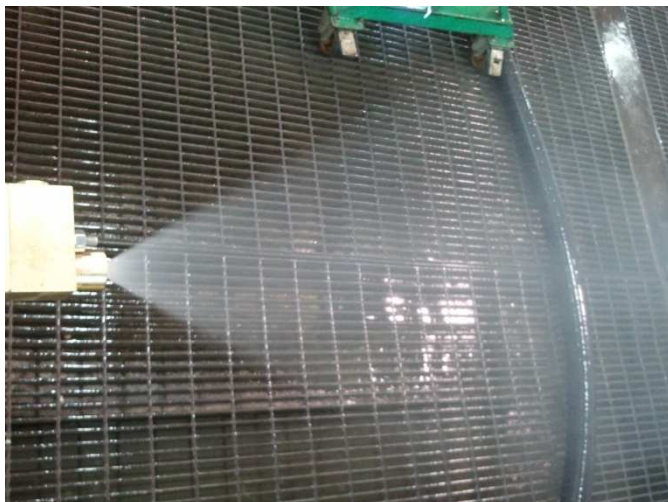
Very uniform hollow cone spray
